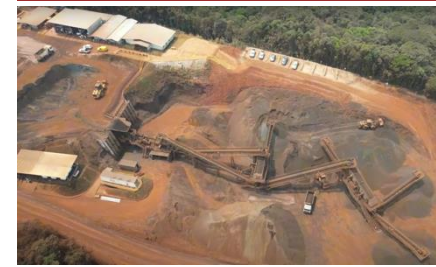
Targeting a dry screening plant similar to Ferro Puro, with dry magnetic circuit whereby test work/existing producers upgrades Fe 10-28% 2
