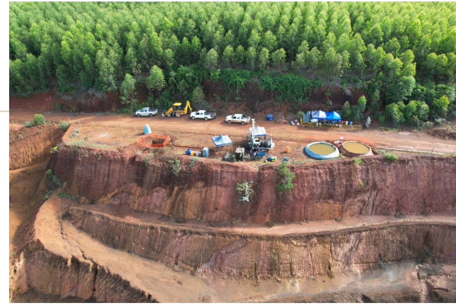
Florália historic open cut (35m face; 160m by 160m) & diamond drilling DH-001 (2025)
